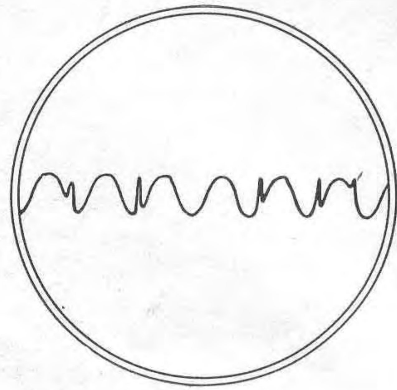
Same signal. Same noise. ANL-ON adjusted for most favorable signal to noise ratio.
